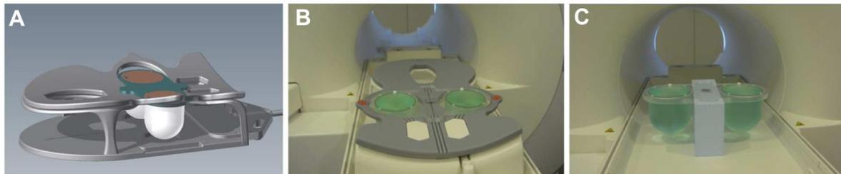
**Fig. 1:** (A) 3D CAD layout of the breast phantom positioned in the RF breast coil. (B) PET scan with the RF breast coil and phantom without insert. (C) PET scan with only the phantom as a reference scan.
