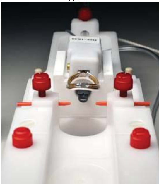
Fig. 1: New coil on top of the 3d printed scaffold inserted into the standard Bruker mouse bed base and tip.
