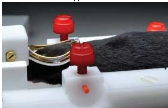
Fig. 2: Placement of the new coil on the mouse head. The copper wire surrounds the head, providing free access to roughly 18mm x 14mm area of the cortex
