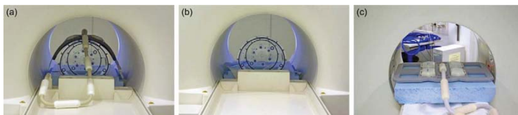
Fig. 1: PET/MR setup. (a) Styrofoam block with the NEMA phantom and the body matrix RF coil was placed in the PET FOV without the patient table. (b) NEMA phantom only used as PET reference scan. (c) Setup of the 511 keV PET transmission scan on an ECAT Exact HR+ PET-only scanner. The flexible RF coil was placed flat on a Styrofoam block.
