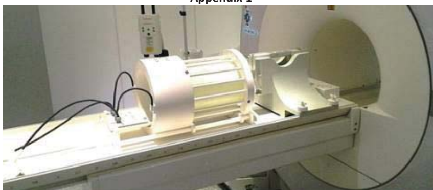
Fig. 1: ^{13}\text{C}/^1\text{H} head birdcage for the 3T Siemens Biograph mMR. Shown is the phantom setup for determining the PET attenuation of the coil. For this, two measurements were performed, once with RF coil (shown) and once without RF head coil (not shown) placed around the active water phantom. Thus, difference maps can be acquired to determine the spatial distribution of PET-signal attenuation.
