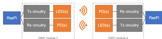
Fig. 9: Schematic of bidirectional communication between two optical wireless module prototypes, PD(s)...photodiode(s), LED(s)...light emitting diodes, RasPi...Raspberry Pi single board computer.
